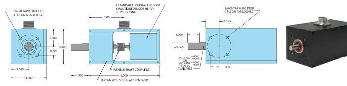
All dimensions are in inches with a tolerance of  $\pm 0.005$ " or  $\pm 0.01$ " unless otherwise specified
