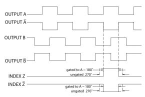
Clockwise rotation as viewed from the mounting face. NOTE: All degree references are electrical degrees. Waveform shown with optional complementary signals.  $\overline{A}$ ,  $\overline{B}$ ,  $\overline{Z}$  for HV output only.
