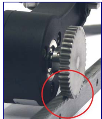
Pinion misalignment can cause inaccuracies or wear.
