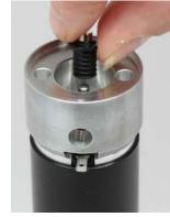
Install Magnet Holder, with magnet in place, over motor's shaft.
