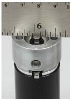
Use a straight edge to ensure magnet is positioned flush with surface.
