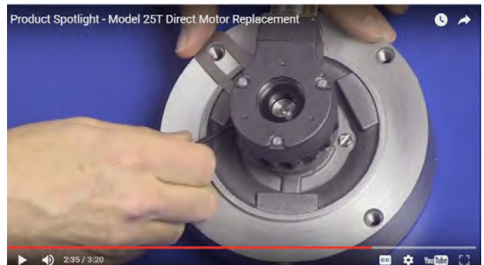
An EPC Model 25T thru-bore encoder, being installed on a motor. For more information, watch the installation video
