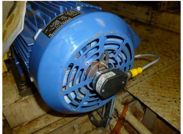
A compact, 2-inch blind hollow bore encoder (1) provides motion feedback on a motor. The flex mount (2) stabilizes the encoder, and the cable sends the electrical signal to the receiver.
