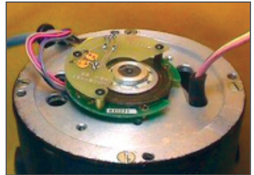
Modular encoder showing sensor and disk
