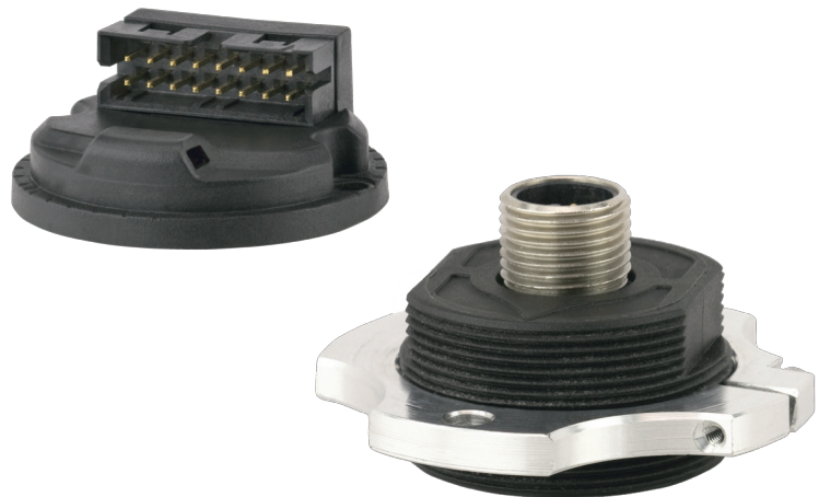
Two examples of magnetic encoder modules. These compact modules are just 30 mm in diameter. The Model 30M (left) is available with 3 different connectors: 8-pin Molex, 16-pin Molex, and an M12 connector. The Model 30MT (right) is a module that includes a threaded housing and an M12 connector. The M12 connectors afford the modules an IP69K seal.
